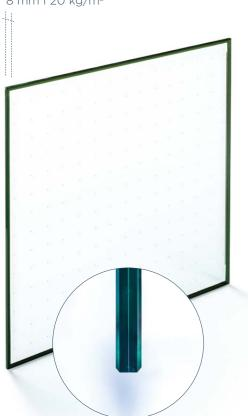
The secret to **FINEO's** exceptional insulating power lies in its structure. Two glass sheets are separated by an extremely thin vacuum cavity of just 0.1 mm.
