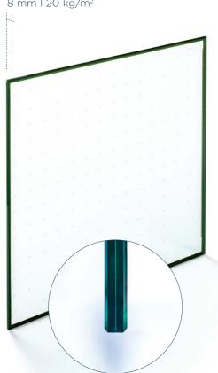
The secret to **FINEO's** exceptional insulating power lies in its structure. Two glass sheets are separated by an extremely thin vacuum cavity of just 0.1 mm.
